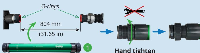
Screw by hand the treatment unit (TU) on the adaptors. Do not use tools, hand tighten only. The arrow must point in the direction of the water flow.
