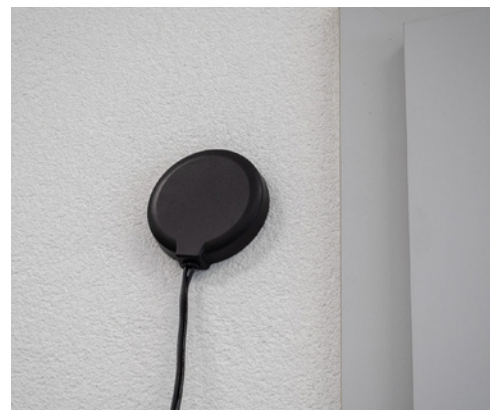
Double sided tape on plaster wall
