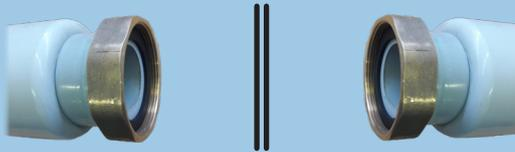
Inspect the treatment unit (TU) and make sure the supplied flat gaskets are in place.
